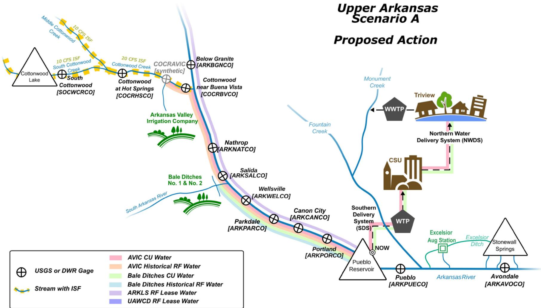
Figure B-5. Upper Arkansas Scenario A Proposed Action Alternative Schematic
