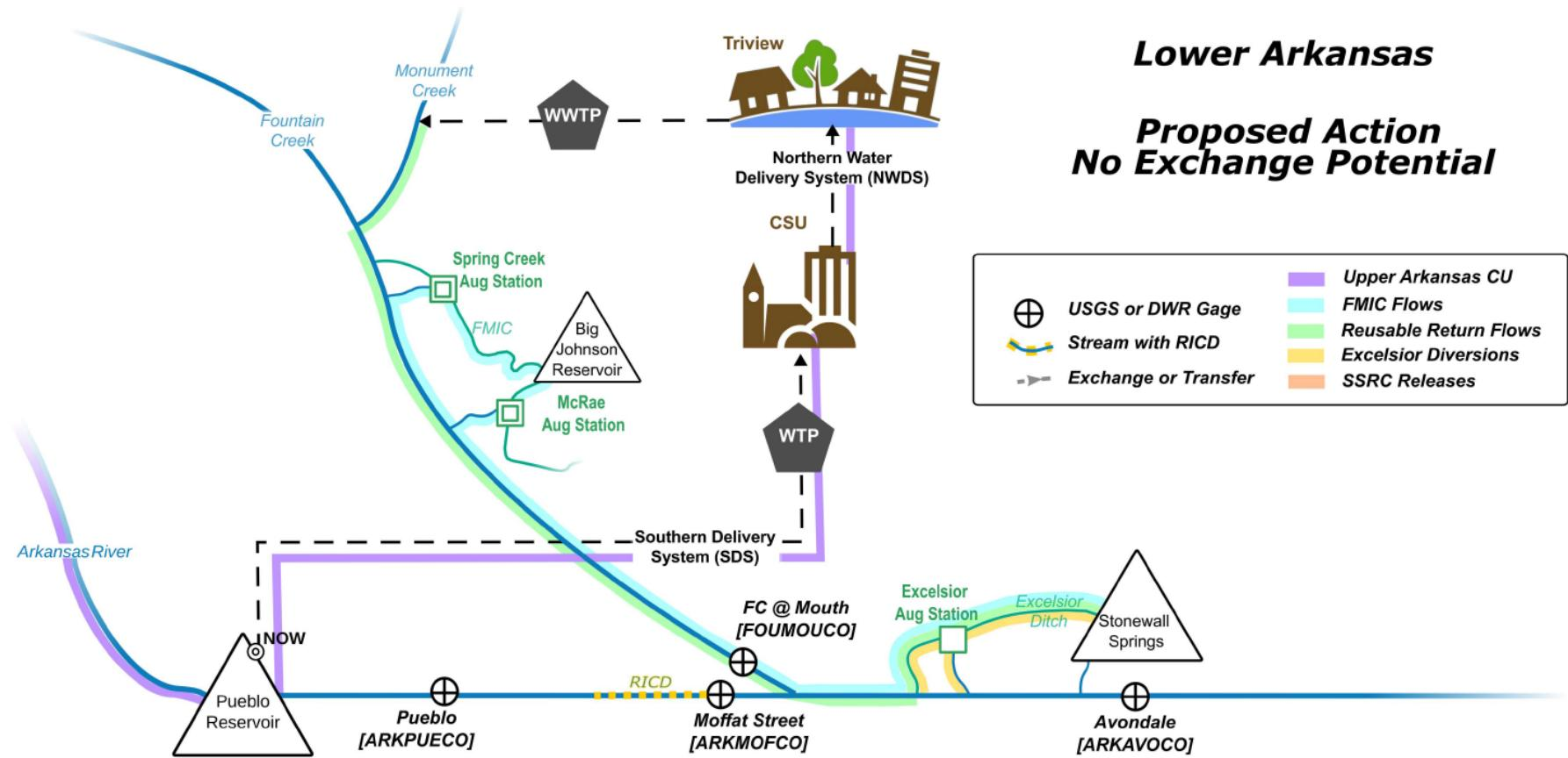
Figure B-7. Lower Arkansas Proposed Action No Exchange Schematic
