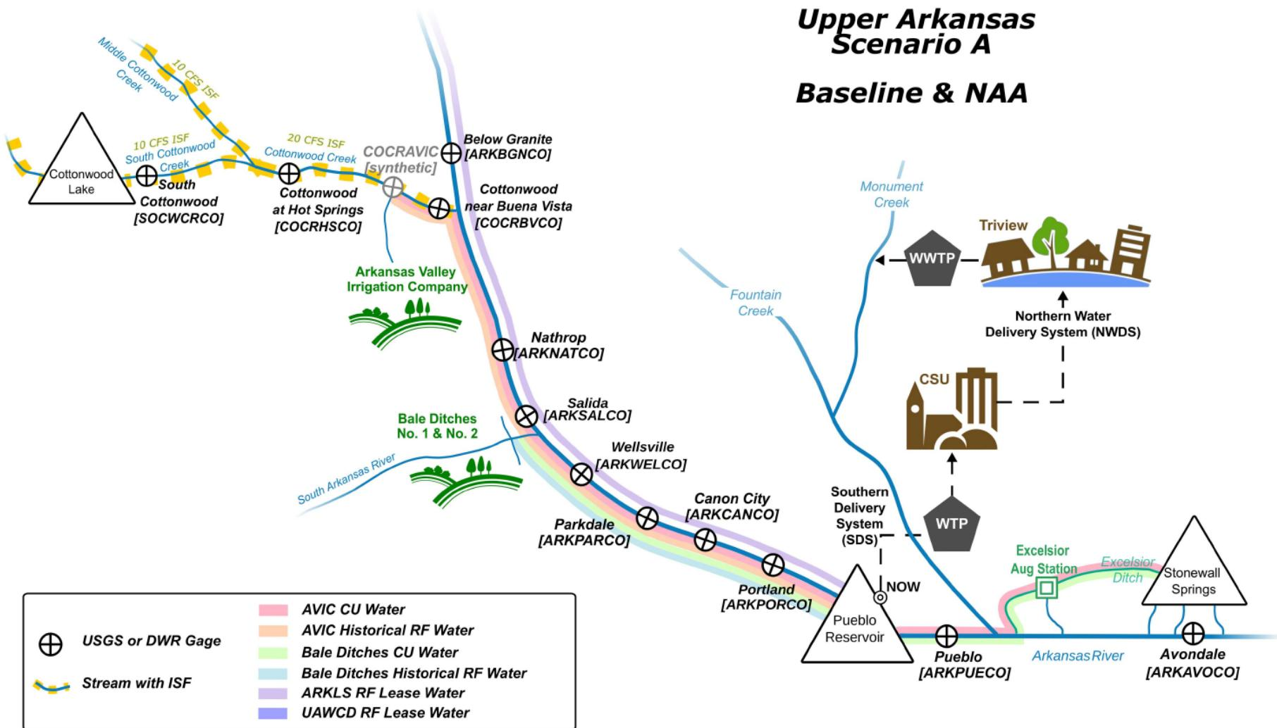
Figure B-2. Upper Arkansas Scenario A Baseline & No Action Alternative Schematic
